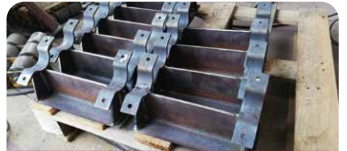
Support ve Kelepçe İmalatı Support & Clamp Bracket Manufacturing
