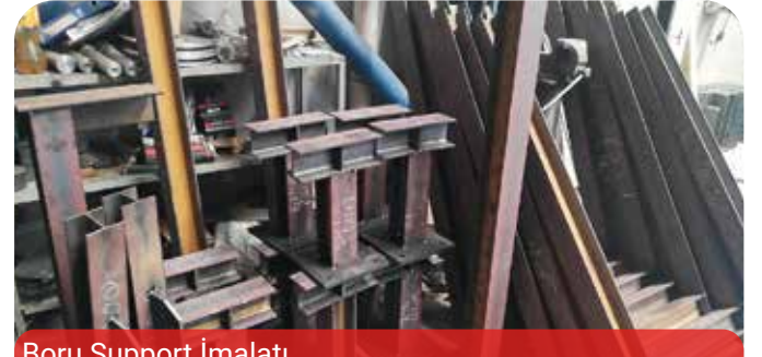
Boru Support İmalatı Pipe Support Manufacturing
